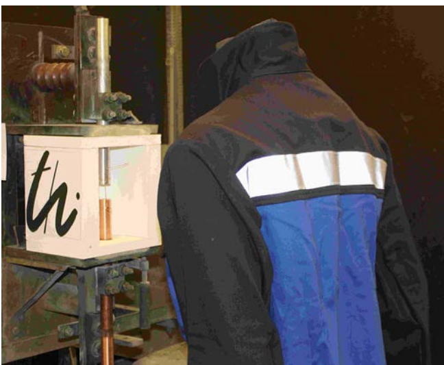
Fig. A 2-1 Test setup, Box test method
