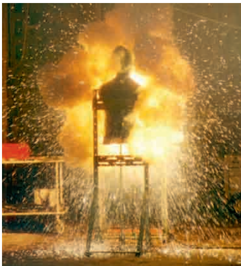
Fig. 5.1: Test mannequin with a jacket exposed to an arc in a box test
