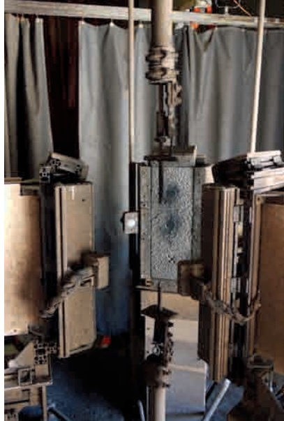
Fig. 5.2: Set-up of the arc rating test (with electrode configuration, sample holders and calorimeter sensors around it)
