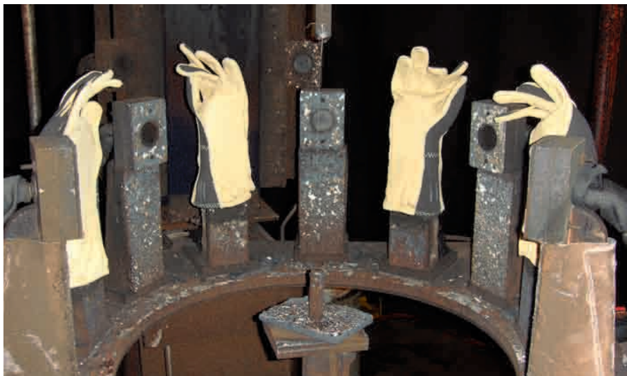
Fig. 7.1: Set-up for glove testing with adapting the arc rating test (source: Dehn+Söhne GmbH + Co. KG)
