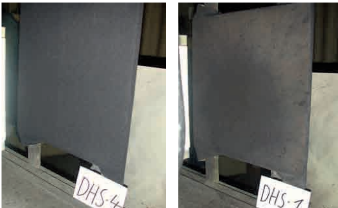
Fig. 5.4: Result of a class 2 box test of a 2-layer textile material system (above) and test sample before testing (below left) and after arc exposure (below right)
