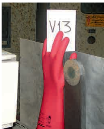
Fig. 7.2: Box test set-up for glove testing with glove panels equipped by calorimeters
