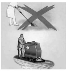
Figure 3: Improper and proper methods for removing flammable dust
