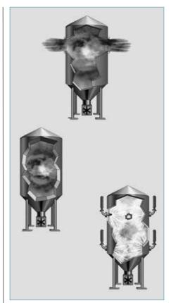
Figure 5: Explosion resistant vessel (left), explosion venting (top) and explosion suppression (bottom right)
