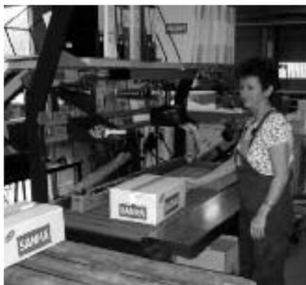
Figure 10: Prevention of lifting and carrying activities through vertically adjustable work tables and roller conveyors
