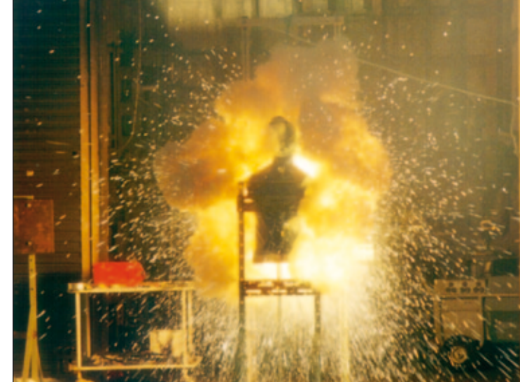
Simulated electric arc in a laboratory for testing of workwear
