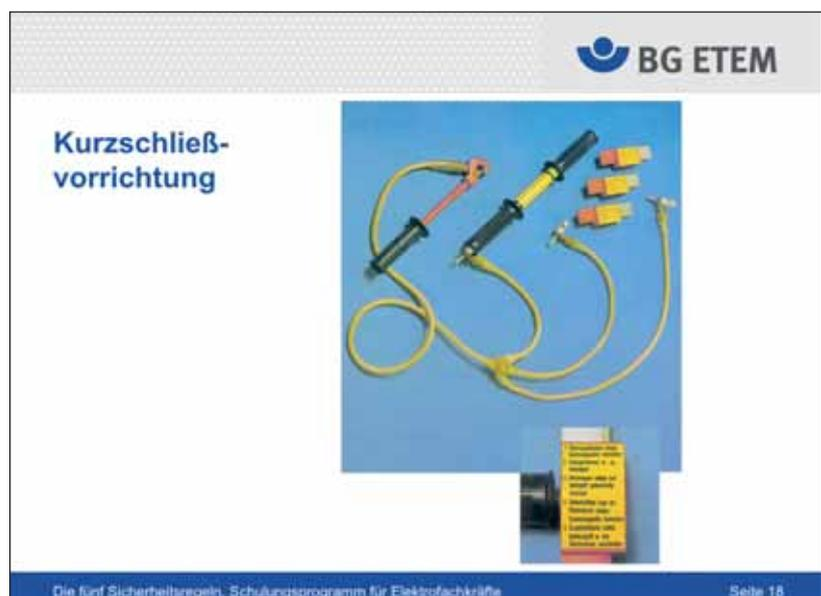
Slide 18: Kurzschließvorrichtung. The slide features the BG ETEM logo in the top right corner. The title "Kurzschließvorrichtung" is on the left. On the right, there is a photograph of a short-circuiting device consisting of two black handles connected by yellow cables, with yellow and red connectors. Below the photo is a small yellow label with text. The footer contains the text "Die fünf Sicherheitsregeln, Schulungsprogramm für Elektrofachkräfte" and "Seite 18".
