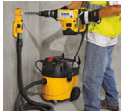
Pictures 3 to 6: Examples of harmonised systems: combi hammers and drill for drilling flush sockets, drilling and chasing with additional collecting unit and a dust-removing unit of Dust Class M
